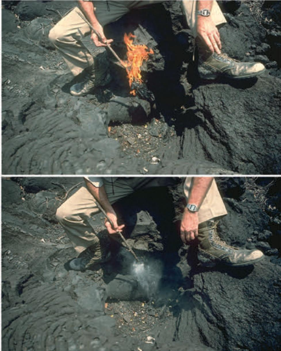
Figure 3. The flame is quickly extinguished when lowered closer to the source of the carbon dioxide (USGS, 2017).
